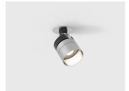
MOD RCSD spotlight with recessed equipment housing (Stefan Diez design). SILVER finishing. Equipped with an interchangeable BLINDER collimator SILVER finishing. Low-voltage head, diameter 100, can swivel through 360° thanks to a nickel-plated copper double hoop. Silver anodised aluminium fin passive heat sink. Interchangeable tubular collimator in silver anodised aluminium
